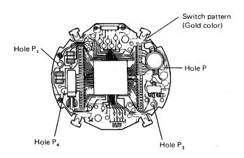
1) The plate complete is positioned by holes  $P_1$  and  $P_2$ .
